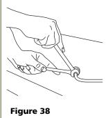
Locate the compression fitting and ferrule packed with the unit. Slide the compression fitting and ferrule over the 1/4-inch OD water supply line. Do not use thread sealing compound or tape. Using two wrenches, tighten the compression fitting on the supply line (see Figure 38).
